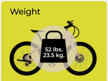
The heavier an object is the more force it takes to move it. Thus, the heavier the load on the ebike the more the motor has to exert itself, the more the motor exerts itself the more power it uses. This all results in a shorter electric bike distance traveled. This isn't only down to the rider's weight but includes the cargo they may be carrying too.
