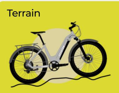
Going uphill requires using more energy as the motor is working against both friction and gravity in this situation, rather than just friction when traveling on flat ground. This is compounded by the weight factor above i.e. more weight going uphill requires even more power. Terrain doesn't just mean hills, and traveling over dirt and gravel, i.e. less grippy surfaces requires more power than traveling on smooth pavements.
