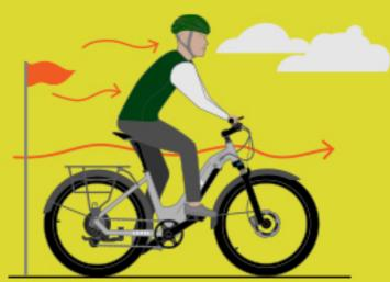
A tailwind can help to buoy you along, assisting you and increasing your range, while a headwind does the opposite, forcing you and your ebike to work harder; thus reducing your range. Wet surfaces, from paved roads to dirt, are also less grippy, meaning that the ebike has to put out more power to push the rider along.
